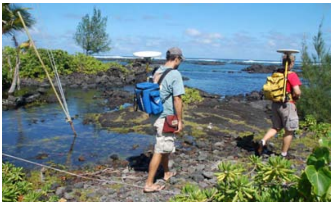
Figure 3-5 – Dual frequency satellite GPS units provide high accuracy in the vertical and horizontal dimension and were used to map the inundation levels for accessible areas.
