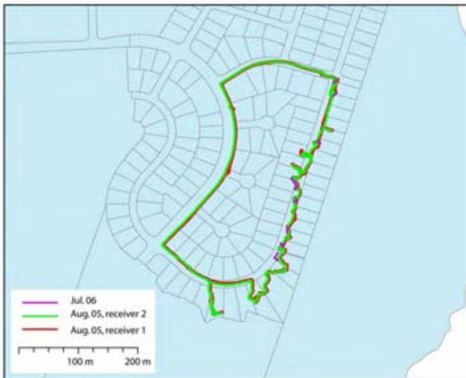
Figure A.6 Street map of Kapolo Vacationlands area with 3 GPS surveys superimposed. Legend indicates the color coding of each survey.
