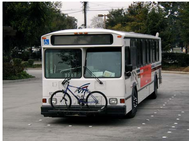
Bike racks on buses provide connectivity between modes. Source: Dan Burden, www.pedbikeimages.org
